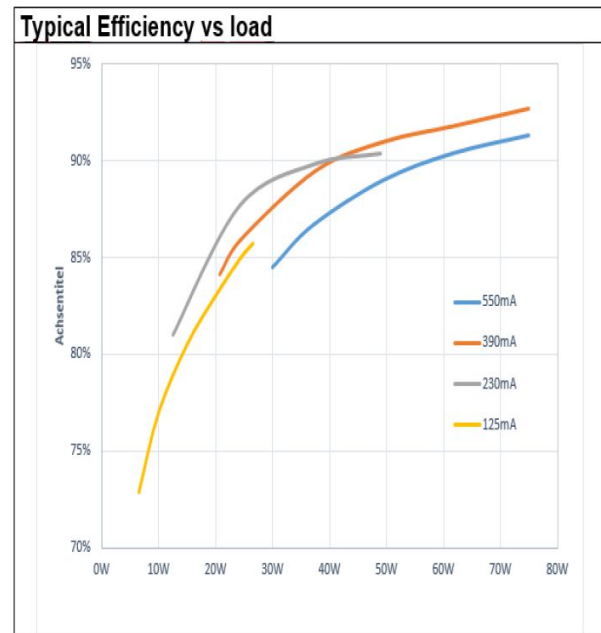
OT FIT 75/220-240/550 D LT2 L Typical Efficiency vs. Load (230 V / 50 Hz)
